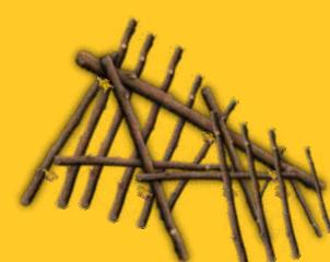
2. Use smaller timbers to create the walls of the shelter, packing them tightly
