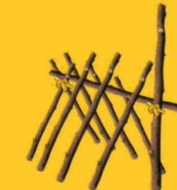
2. Using smaller lengths of timber, build up the walls ensuring timber is tightly packed
